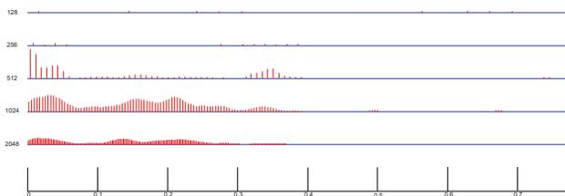
**Fig. (7).** The sound of Fig. (6c) after Daubechies wavelet transform; smoothed absolute values of the transformation coefficients for five different scales. They can be directly used for building a searchable feature vector of this heart sound.
